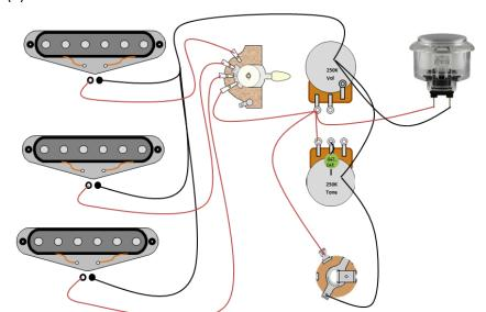
Wiring your Tesi DITO kill switch is simple. Take the red wire and connect it to the hot or live signal on your volume pot. The Black wire can be connected to any ground point within the guitar.
